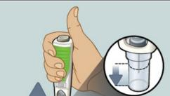
Lift the pen straight up from the skin. The needle guard on the tip will automatically move down to
